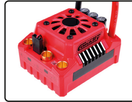
C-54011 Speed Controller - TOROX 185 - Brushless - 2-6S
