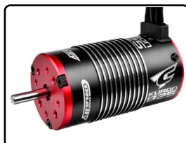
C-54055 Brushless Motor - Kuron 825 - 4-Pole - 2050 KV - Sensorless
