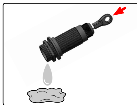
Drain the oil from the shock absorber.
